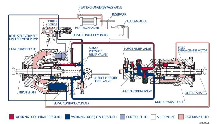
Above figure shows schematically the function of a hydrostatic transmission using an axial piston variable displacement pump and a fixed displacement motor.
