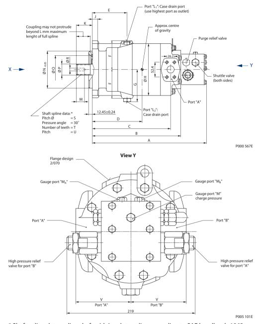
\* Shaft spline data: spline shaft with involute spline, according to SAE handbook, 1963, class 1, fillet root side fit.
