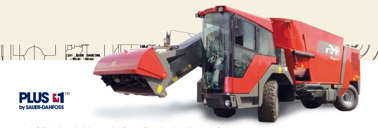
speed of 40kph when unloaded – twice that of conventional tractor-pulled mixer feeders. Series 90 pumps also supply hydraulic flow to the chopper and mixer motors.
