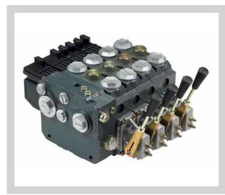
PVG 100 is a load independent proportional valve with flow up to 180 l/min [48 gpm] and pressures up to 350 bar [5076 psi]. It offers equitable flow sharing for precise control of multiple machine functions under varying load conditions and pressure requirements.
